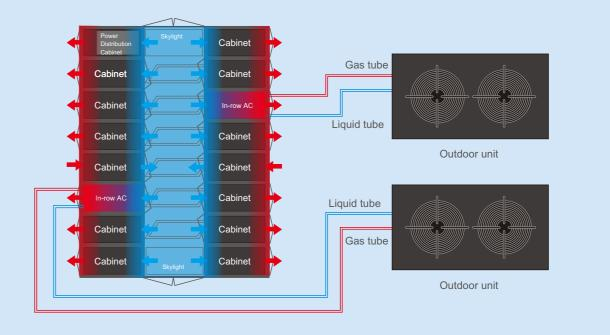
When the outdoor unit is higher than the indoor unit: the vertical height difference between indoor and outdoor units should not exceed 20m; when the indoor unit is higher than the outdoor unit: the vertical height difference between indoor and outdoor units should not exceed 5m.
